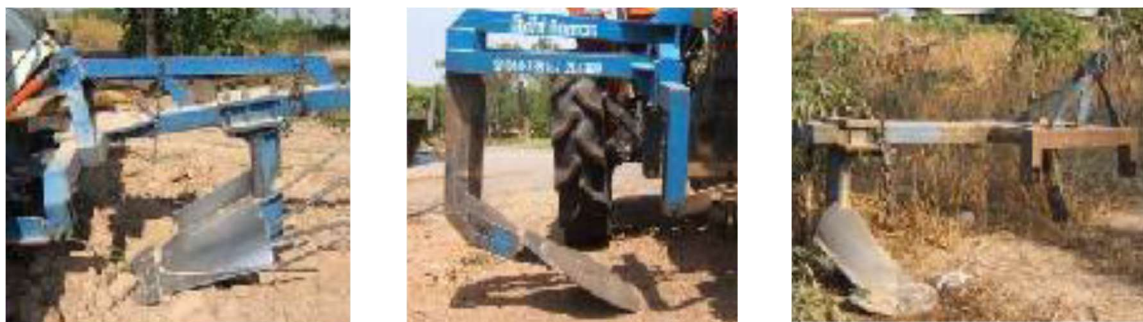
Figure 7 Type of cassava diggers available in Thailand (Chamsing et al. , 2012).
