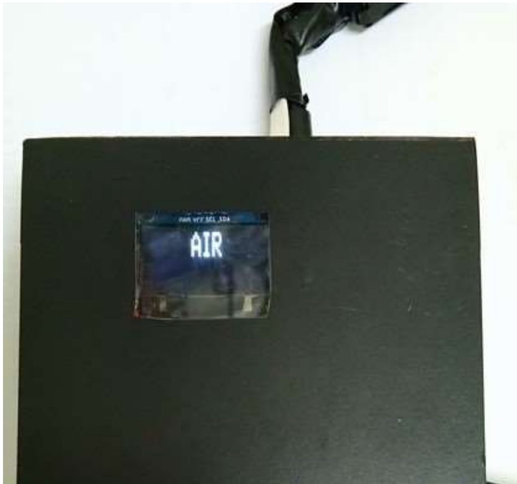
Figure 3 Alerted information on the air bubble detected system case
