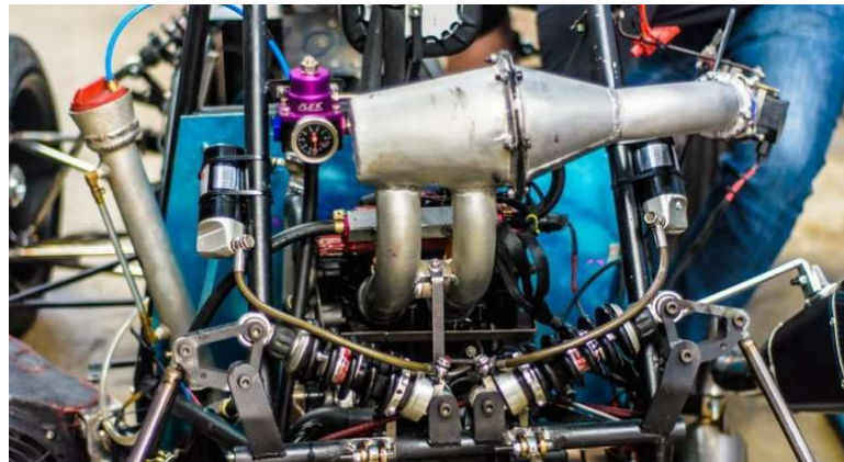
Figure 8 Final implementation of the engine intake manifold in the racing car.
