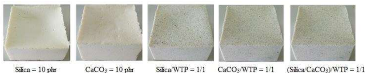
Figure 10 Photographs of filler and WTP - filled NRLF
