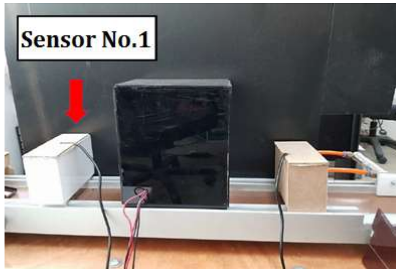
Figure 8 Sensor No.1 stand by detects moving coins.
