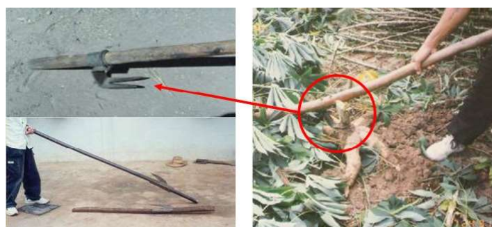
Figure 5 An indigenously developed Cassava lifter by Thai farmers (Mac hoe). (Mongkol et al. , 2007)
