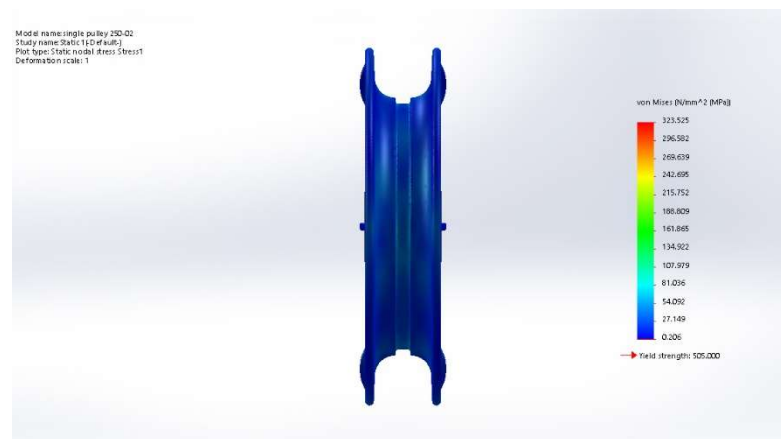
Figure 12 von Mises stress Case Study 2, Right View
