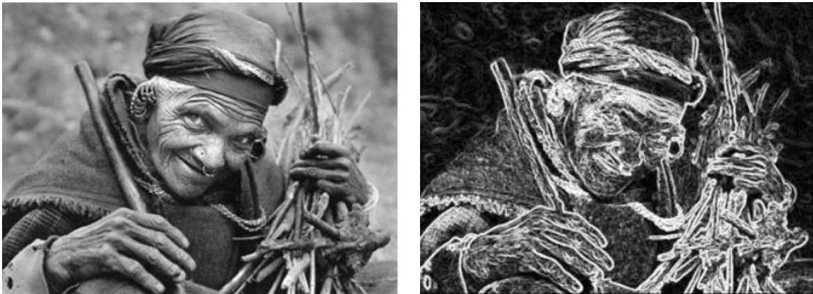
Figure 4 The example of finding edge by the Sobel method (Gonzalez and Woods 2002)
