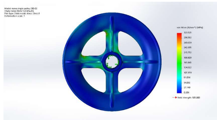
Figure 11 von Mises stress Case Study 2, Front View
