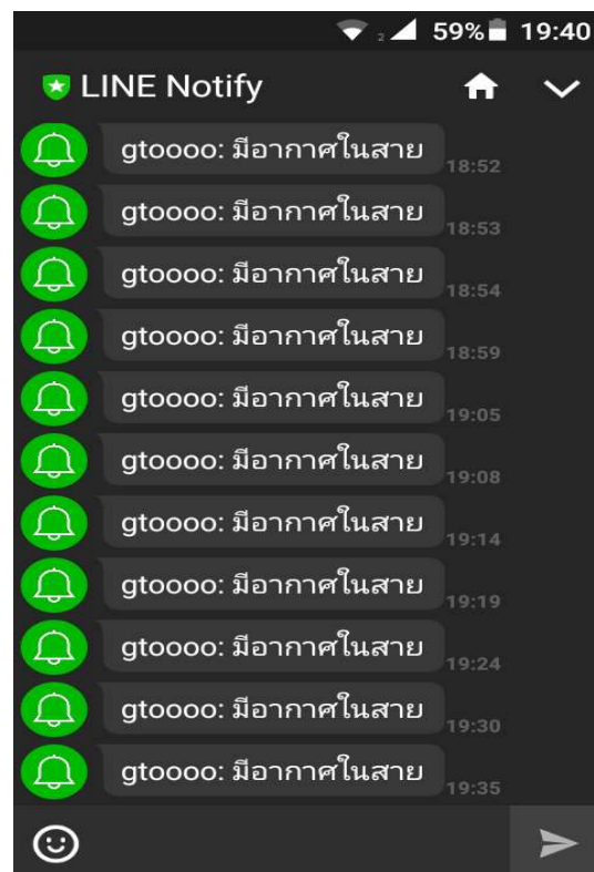
Figure 5 LINE application shown warning message that there is air bubble in IV tube.
